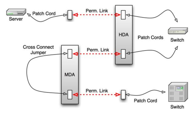
ISO/IEC and TIA standards define Link testing to verify the performance of the fixed (permanent) segments of installed cabling as accurately as possible.
