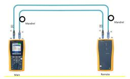
2. After referencing (Results between -22dB and -24dB for MM and -6dB and -8dB for SM). Add LC to LC reference cords and test them to ensure they are less than or equal to 0.15dB standard for IL for MM and 0.25dB or less for SM). Save the test result as Ref 1, Ref 2. If you re-reference for any reason, resave the values as Ref 3, Ref 4...etc...until testing is complete.
