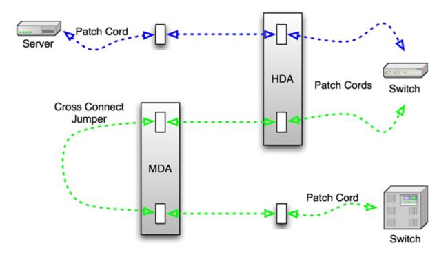
Ultimately, network functionality and signal integrity relies on the performance of the Channel (the completed end to-end link). Installation and test personnel do not typically measure end-to-end loss of the complete Channel with all EDA cords and cross connect cables in place.
